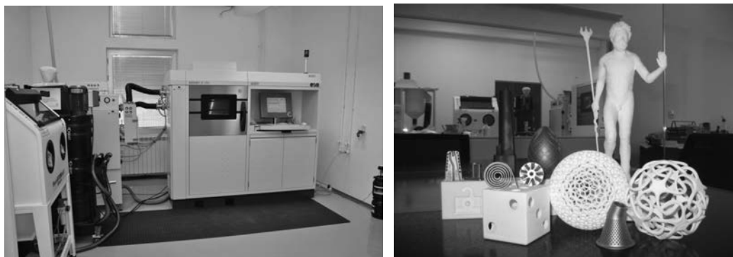
Fig. 4 Laser sintering machine and some products made in "3D Impulse"
